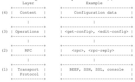
Figure 1 illustrates how NETCONF may be conceptually partitioned into logical layers. This is in fact an excellent architecture for our purpose. It mirrors the actual protocol and minimizes the degree of coupling between the different layers.
